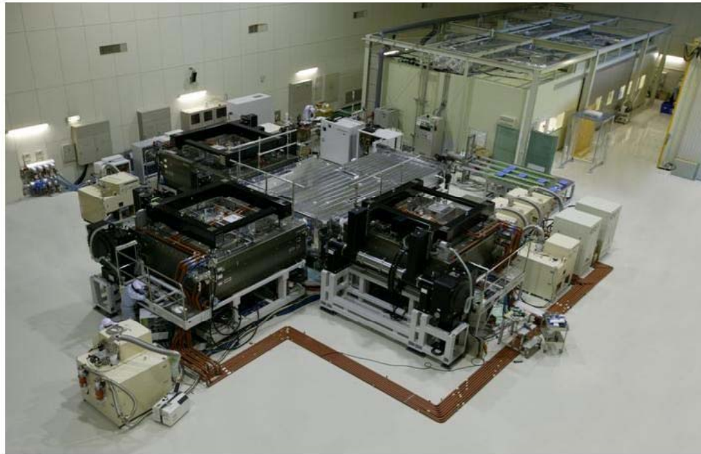
G7 Plasma Dry Etching System (3-chamber type)
