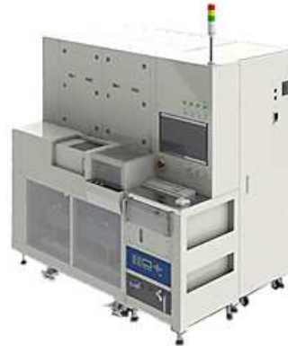
Backside Laser Annealing System for Ohmic Contact Formation on SiC
