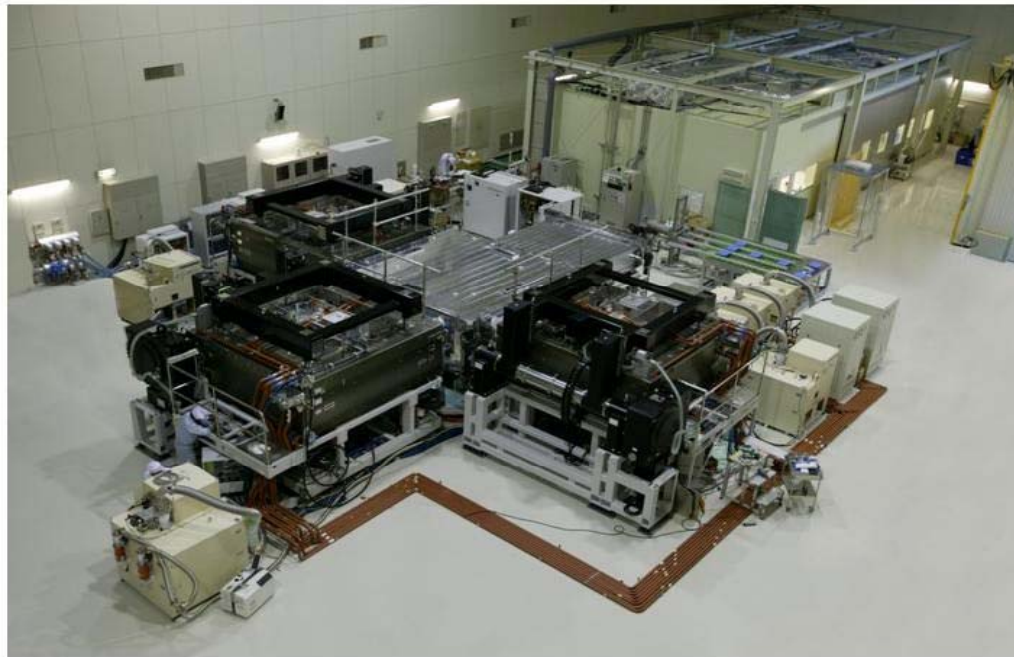
G7 Plasma Dry Etching System (3-chamber type)
