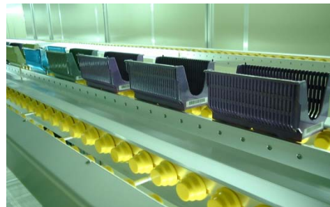
Clean Conveyor (for Hard Disk Factories)
