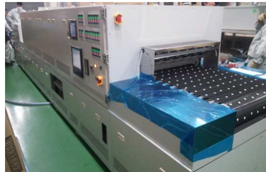
Consecutive muffle kiln with mesh belt conveyor
