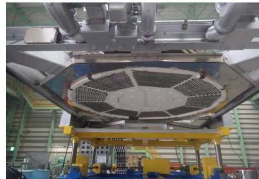
Large forging heat treatment equipment for aircraft
