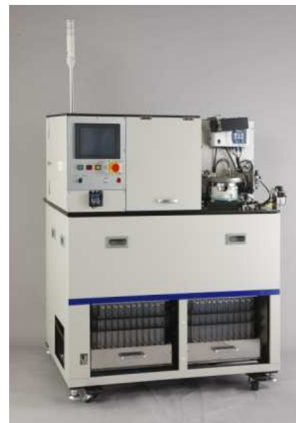
Inspecting and sorting machine for SMD-LED
