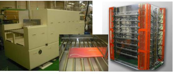
Tempering equipment for high tension sheet steelRoller-Hass typeVertical heater
