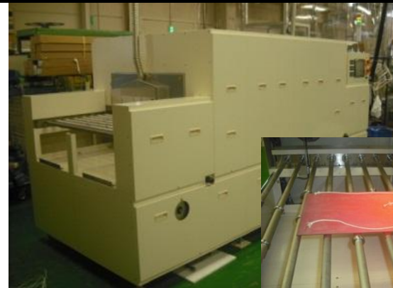
Tempering equipment for high tension sheet steel Roller-Heater type
