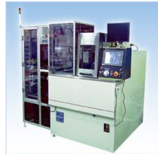
DAR810 Full automatic core drilling machine
