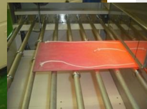
Tempering equipment for high tension sheet steel Roller-Heater type
