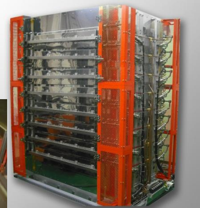
Tempering equipment for high tension sheet steel Roller-Heater type
