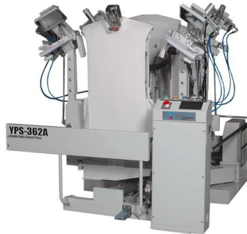
Body-sleeve pressing machine for
