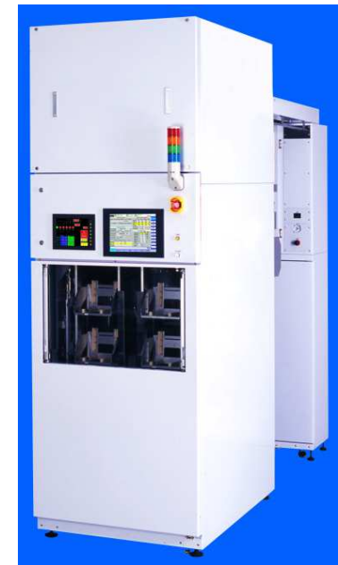
Vertical diffusion furnace Semiconductor manufacturing equipment
